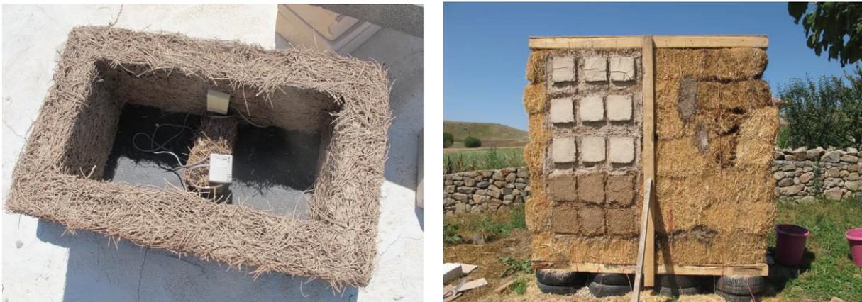
Figure 10. Academic research and experiments on building materials and their properties include the study of lightweight loam and pine-needles (left) and applying different types of mud plaster on straw bale walls to assess their durability (right).
