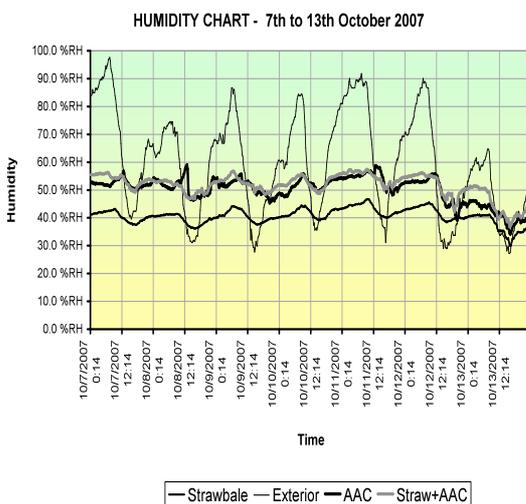
Fig 6. Humidity readings from the three buildings and external humidity levels during a 7 day period in October 2007
