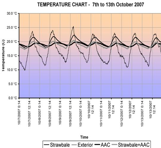
Fig 5. Air temperature readings from the three buildings and external air temperature during a 7 day period in October 2007
