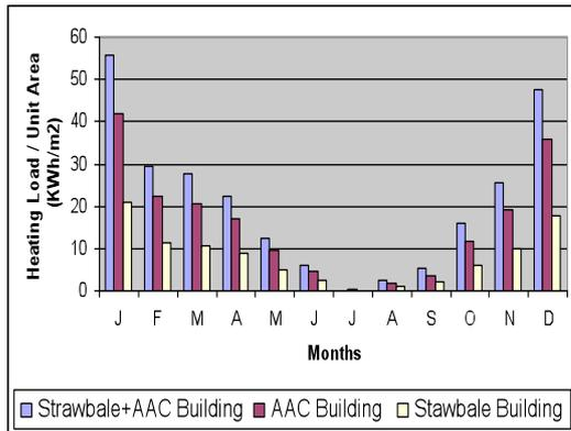
Fig 7. Comparing simulated monthly heating/ cooling loads for the three buildings shows strawbale to be the most energy-efficient building material.
