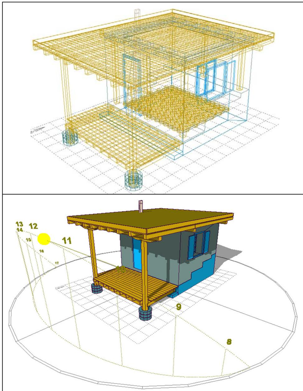
*Figure 16. The basic 3D model (above) in Ecotect v.5.20 is then rendered and shaded (below) for more realistic visualisation of shading analysis with the sunpath diagram on a particular date and time for the geographic location of Yozgat.*
