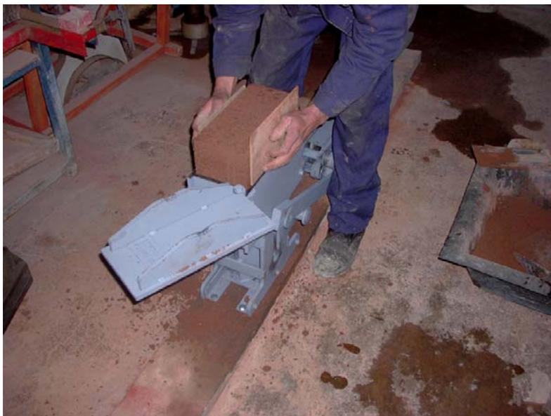
*Figure 6. Once pushed up the brick can be taken out by holding it with two plywood pieces to avoid damage. The bricks are then stacked for drying.*
