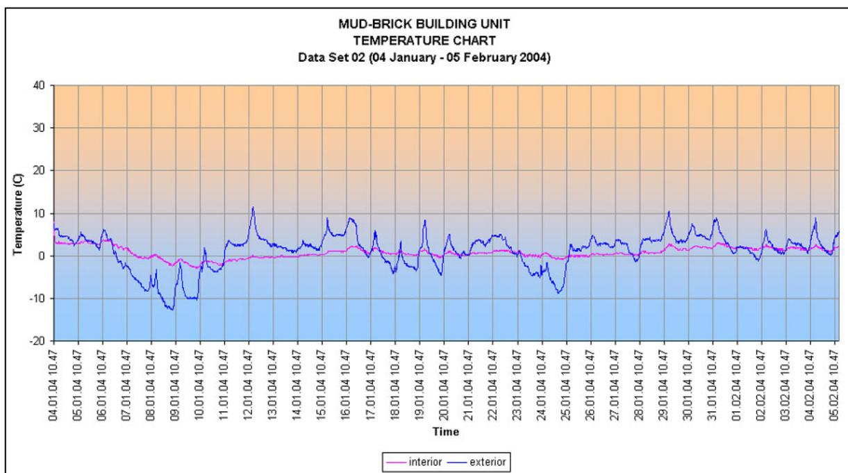
*Figure 19: Diurnal range of indoor temperature (shown by pink lines) for the mud-brick building plotted against outdoor air temperature (shown by blue lines) for one-month period between 04 January and 05 February 2004 during which the building was neither occupied nor heated.*
