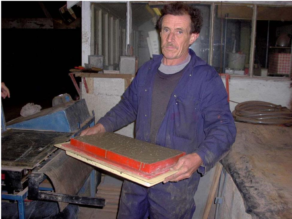
*Figure 10. Moulds for the similar production of different types of roof tiles and paving slabs are also available.*
