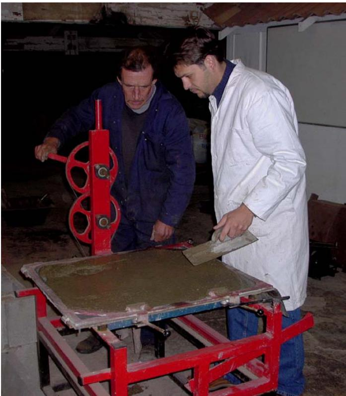
*Figure 8. The Human powered Parry's Multivibe Vibrating Table can also be connected to the electricity circuit. De-aerating the concrete mix by means of vibrations will strengthen the product and reduce the thickness required.*
