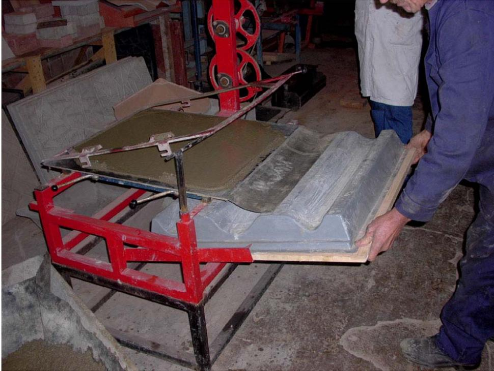
*Figure 9. The plastic sheet on which the cement mix was poured can be pulled over the roof tile mould. Up to 20 moulds can be stacked for drying.*
