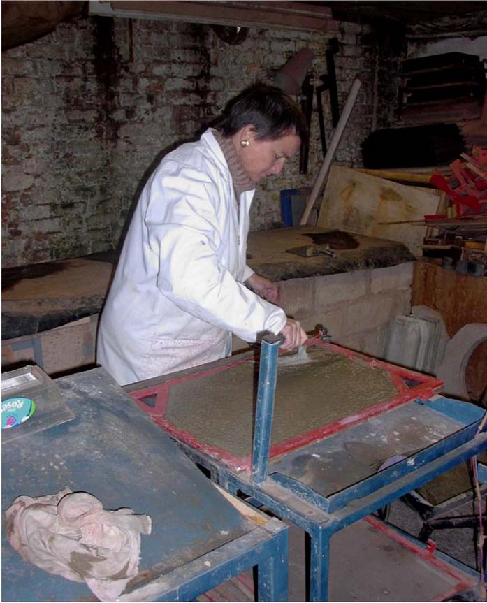
*Figure 7. Production of micro cement building elements in a small workshop will not require a large capital investment.*
