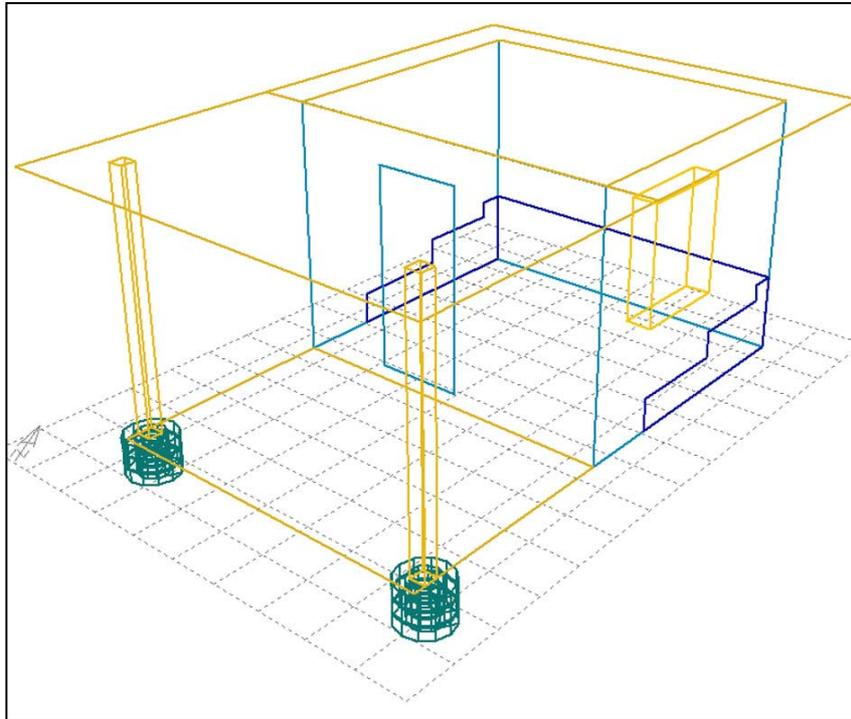
*Figure 17. A 3D view of the thermal model of mudbrick building developed in Ecotect v.5.20.*
