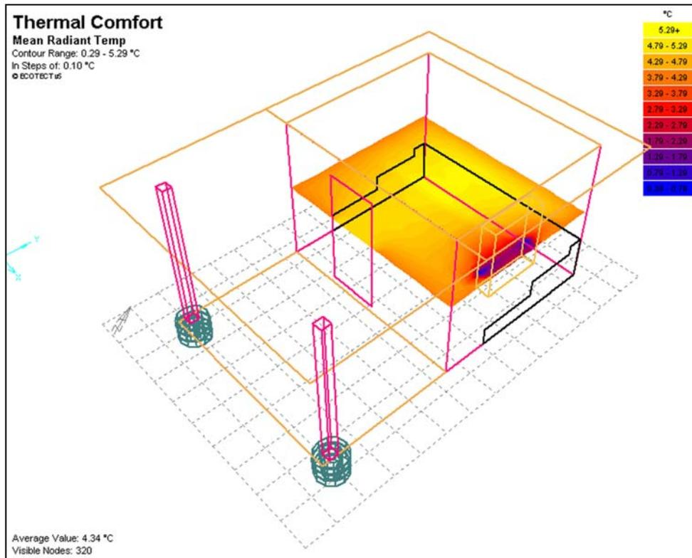
Figure 23: Results of the thermal analysis performed with Ecotect v.5.20 showing the mean radiant temperature levels shown (colour scale ranging from 5.29 °C to 0.29°C) on a grid inside the mud-brick building for the 20<sup>th</sup> of January 2004 under the climate conditions of Yozgat. The building is assumed to be unoccupied and there is no air-conditioning system in operation.
