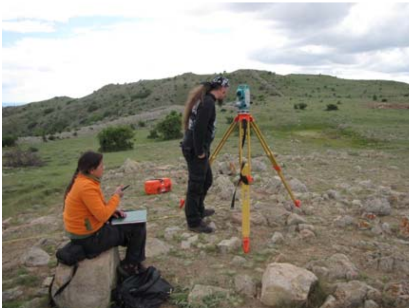
Figure 42. Güzin Eren and Ferhat Can using the total station to relocate unmarked grid corners for the electrical resistance survey. (10dpcp0614)
