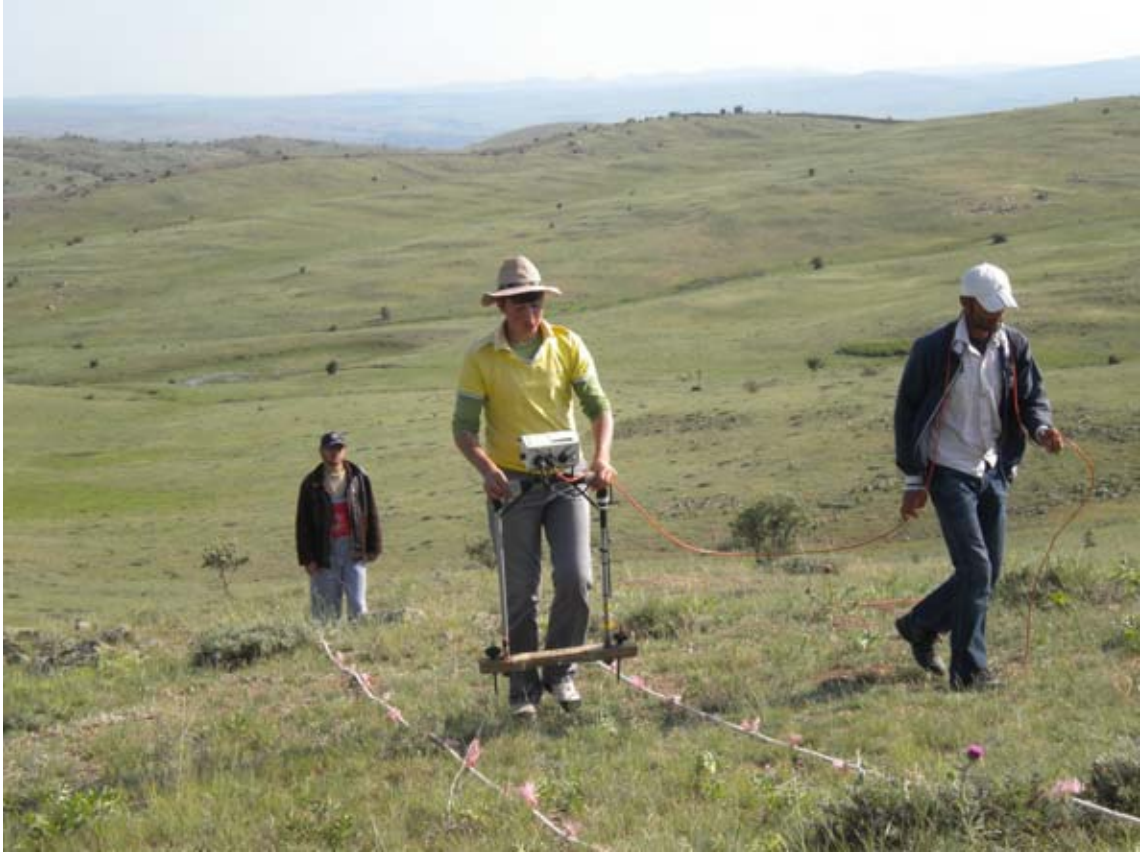
Figure 55. Electrical resistance survey of the 'Temple' area by a team of three, Cafer Babayiğit, Muhammed Babayiğit and Mehmet Baştürk. (10dpkc0111)
