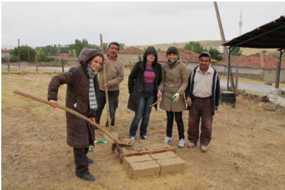
Figure 12. Students learn from villagers how to produce traditional mudbricks. (10kecg0611)
